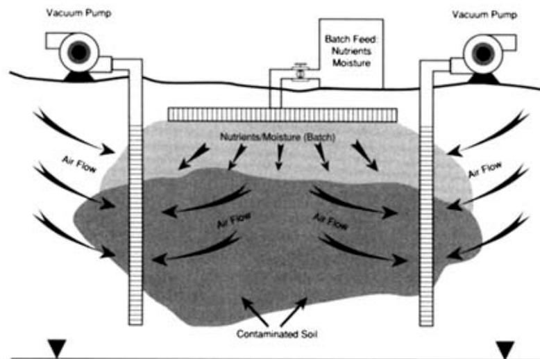
**Fig. 2:** In-situ bioremediation by applying engineering measures (Tyler, A., *et al.*, )
