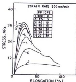
**Fig. 7:** Stress-strain curves of PP/CPE blends at a strain rate of 500 mm/min
