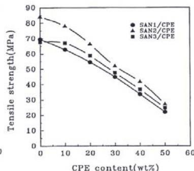
**Fig. 6:** Tensile strength versus composition
