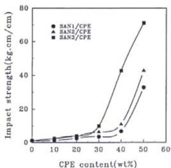
**Fig. 4:** Notched Izod impact strength versus composition
