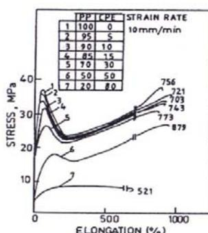
**Fig. 8:** Stress-strain curves of PP/CPE blends at a strain rate of 10 mm/min
