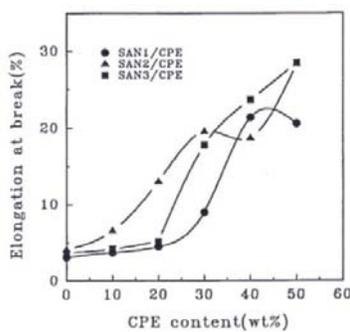
**Fig. 5:** Elongation at break versus composition
