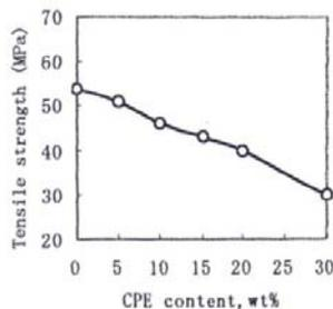
**Fig. 2:** Tensile strength versus composition
