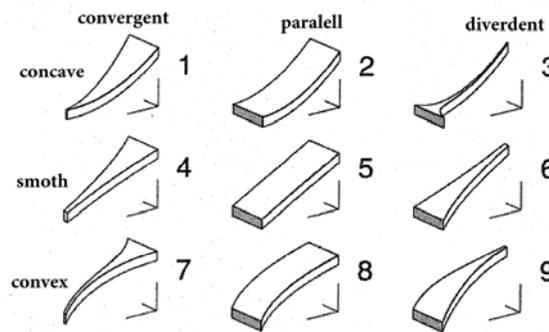
**Fig. 3:** Hydrology shape of the slope
