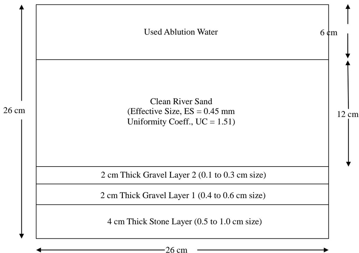
**Fig. 3:** Schematic Section of the Lab-scale Sand Filter (Not to Scale)
