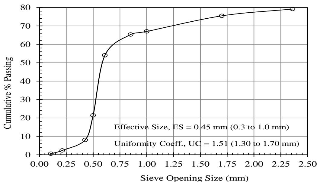
**Fig. 2:** Characteristics of the Sand Filter Media used for the Lab-scale Filter
