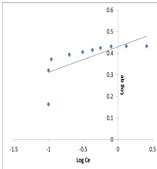
Fig. 12: Freundlich model “ $\text{Log } q_e$  vs.  $\text{Log } C_e$ ” for Fe
