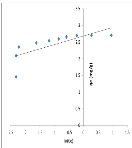
Fig. 13: Temkin model “ $q_e$  vs.  $\ln(C_e)$ ” for Fe
