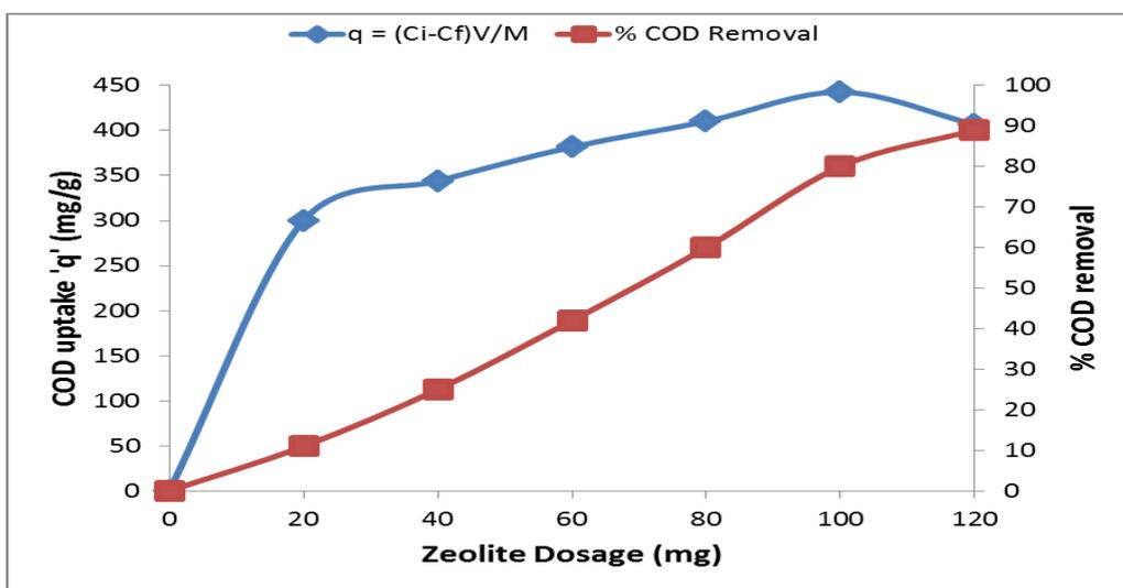
Fig. 5: Effect of zeolite dose on COD uptake.
