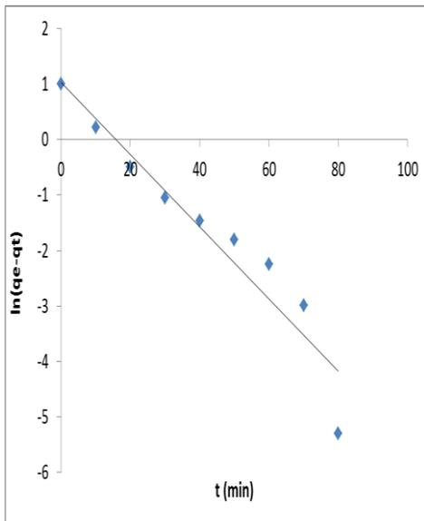
Fig. 19: Pseudo-first-order model “ $\ln(q_e - q_t)$  vs.  $t$ ” for Fe
