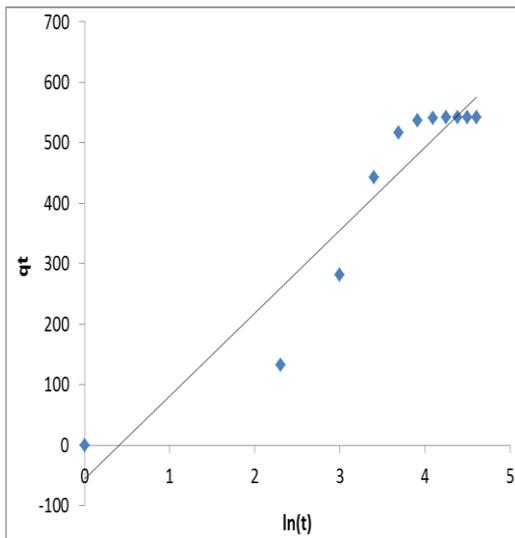
Fig. 17: Elovich model “ $q_t$  vs.  $\ln(t)$ ” for COD
