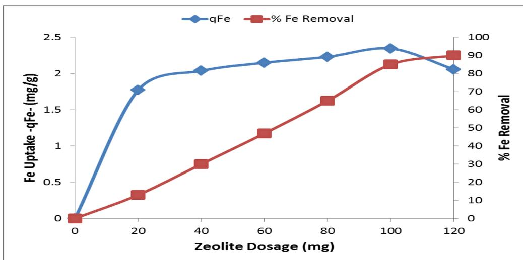
Fig. 6: Effect of zeolite dose on Fe uptake.
