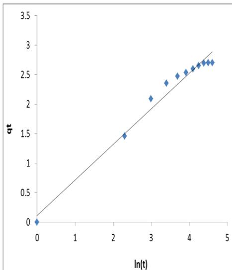
Fig. 21: Elovich model “ $q_t$  vs.  $\ln(t)$ ” for Fe
