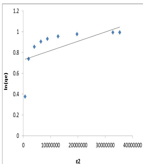
Fig. 14: D-R model “ $\ln(q_e)$  vs.  $\epsilon^2$ ” for Fe
