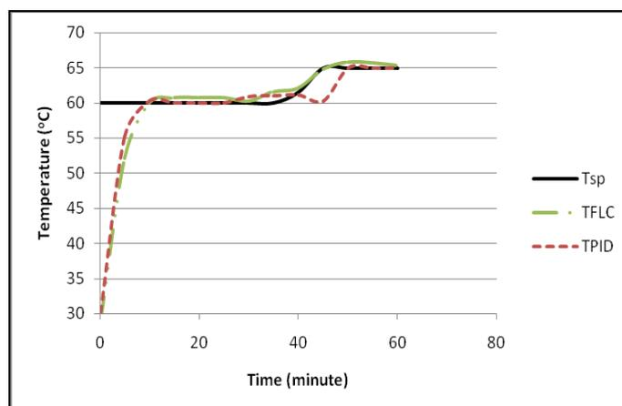
**Fig. 1:** Performance of Fuzzy Logic controller (pH=8, 150 rpm,  $E_t=12 \text{ gmL}^{-1}$ ).
