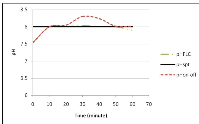
**Fig. 2:** Performance of pH control using Fuzzy Logic controller ( $T=60^{\circ}\text{C}$ , 150 rpm,  $E_t=12\text{ gL}^{-1}$ , batch reactor)
