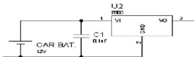
Fig. 4: Voltage regulator schematic diagram
