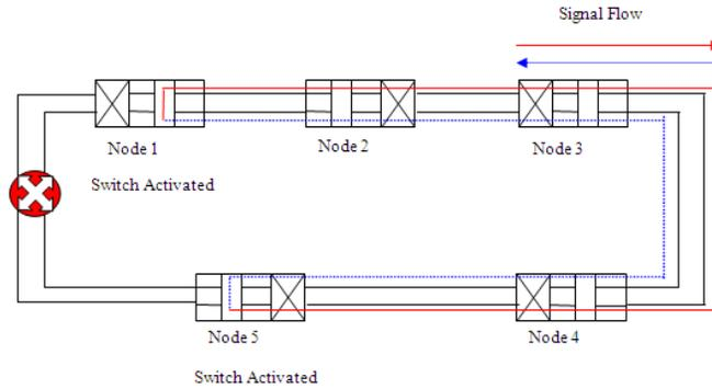
**Fig. 6:** Ring protection mechanism is also used for recovery for odd number of nodes in optical ring network when both lines fail.
