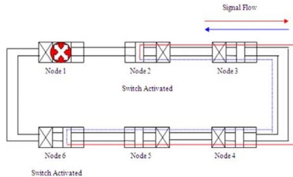
**Fig. 5:** Ring protection mechanism is activated to quarantine the failure/node area from the working area by rebuilding the new ring network.
