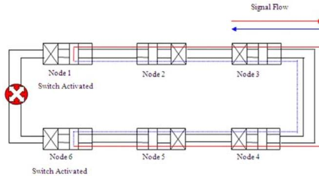
**Fig. 4:** Network recovery for the case of failure occurs at the both lines by using ring protection. Node 1 and Node 6 activate ‘U’ turn switch when received emergency signal from the nearest node to the failure area.
