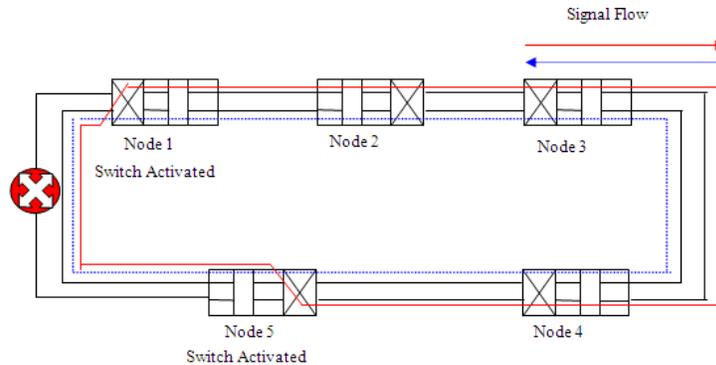
**Fig. 7:** Linear/Multiplex protection mechanism is also used for recovery for odd number of nodes in optical ring network when one of the lines fail.
