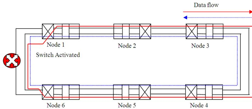
**Fig. 2:** Network recovery for the case of failure occurs at the working line by using linear/multiplex protection. Node 1 and Node 6 activate path change switch when received emergency signal from the nearest node to the failure area.
