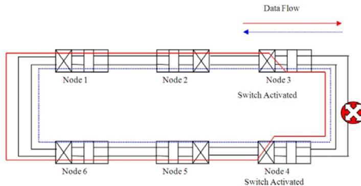
**Fig. 3:** Network recovery for the case of failure occurs at the working line by using linear/multiplex protection. Node 3 and Node 4 activate path change switch when received emergency signal from the nearest node to the failure.
