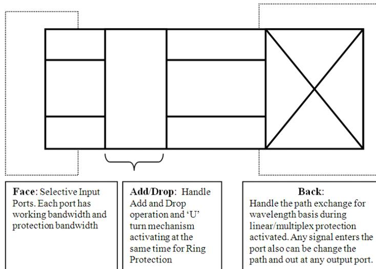
**Fig. 1:** OXADM node symbol and classification based on the function and mechanism.
