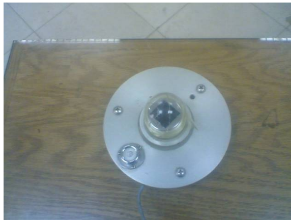
Fig. 8: Athermopile pyranometer of type Kipp & Zonen model.
