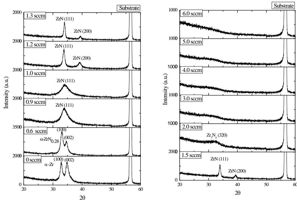
**Fig. 1:** X-ray diffraction patterns for Zr-N films deposited with various  $N_2$  flow rates at Zr current of 0.6 A and deposition time of 15 minutes.
