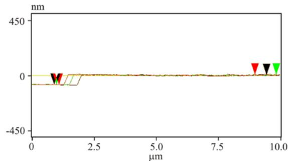
**Fig. 3:** Section analysis of zirconium nitride films at a constant sputtering current of 0.6 A and a deposition time of 15 min.
