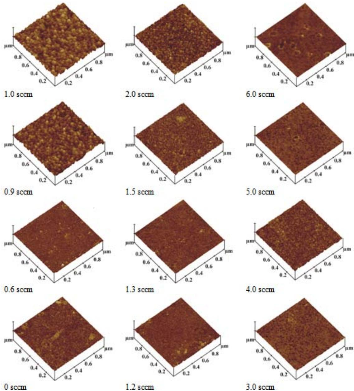
**Fig. 2:** Surface morphologies of zirconium nitride films (3D images) deposited with various N<sub>2</sub> flow rates at Zr current of 0.6 A and deposition time of 15 minutes.
