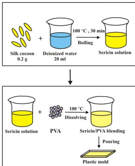
**Fig. 1:** Schematic of the extraction of sericin solution and the preparation of sericin/PVA hybrid film
