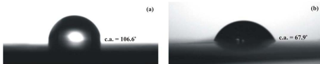
**Fig. 3:** Photographs of contact angle for (a) PVA film and (b) sericin/PVA hybrid film
