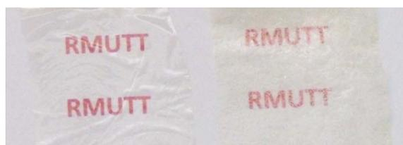
**Fig. 2:** sericin/PVA hybrid film (left) and sericin/ PVA film loaded with amoxicillin trihydrate (right)
