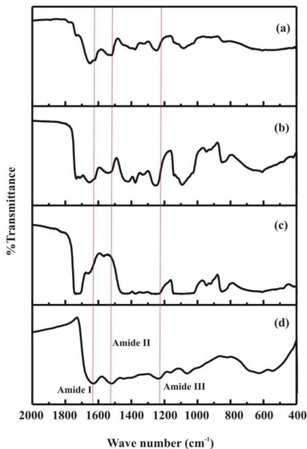
**Fig. 4:** FTIR spectra of (a) silk cocoon, (b) PVA film, (c) sericin/PVA hybrid film and (d) sericin/ PVA film loaded with amoxicillin trihydrate
