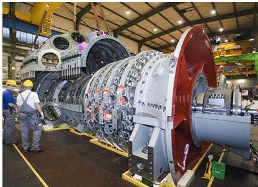
Fig. 3: H-class gas turbine (courtesy of Siemens)
