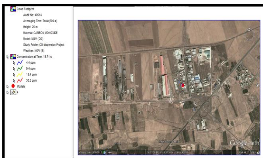
Map. 1: Top view of emission of CO gas from stack of Takestan Steel Factory at stack level in November
