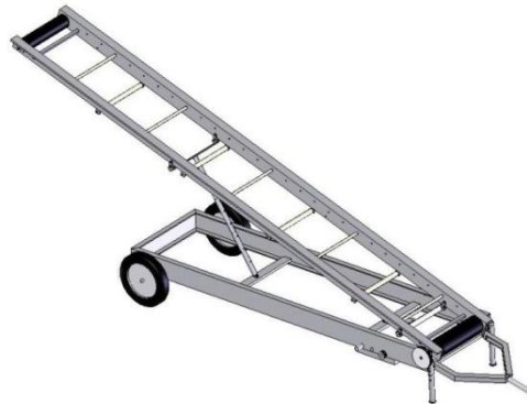
Fig. 11: A view of the Conveyor Belt Lift (the conveyor belt is not shown)
