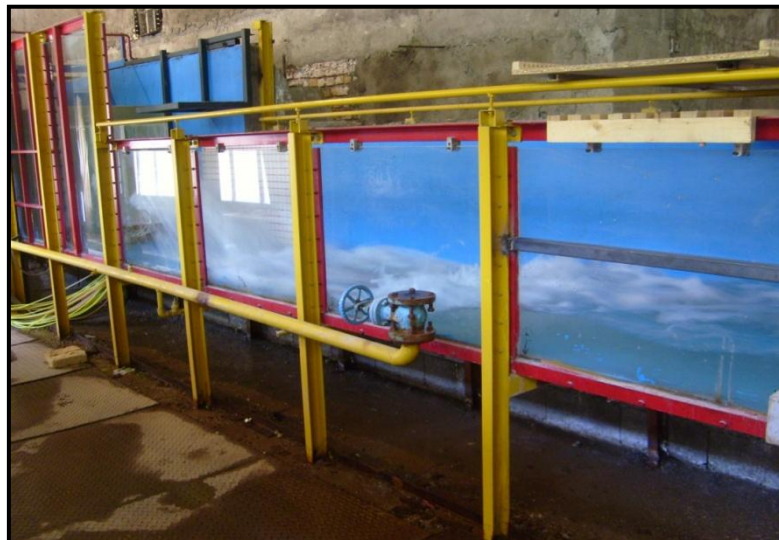
Fig. 2: Constructed experimental flume
