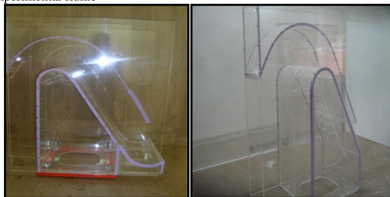
Fig. 3: Constructed siphon from Perspex material
